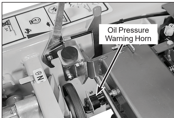
Warning Horn Location
