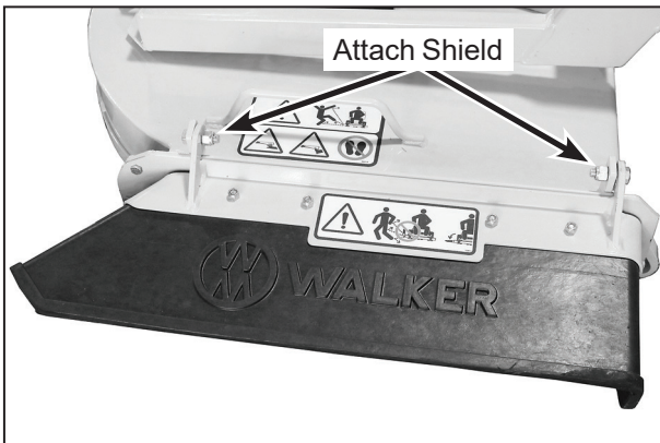
Discharge Shield Installation on Side Discharge Deck
