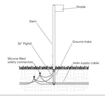
The operating voltage range for this LED luminaire is 6 - 15 volt AC. The Vista electronic driver ensures the LED operates at the intended lumen output while receiving voltage as low as 6 volts, and as high as 15 VAC, resulting in a balanced lumen output from the first fixture to the last. Eliminating the dimness issues often attributed to voltage drop.
