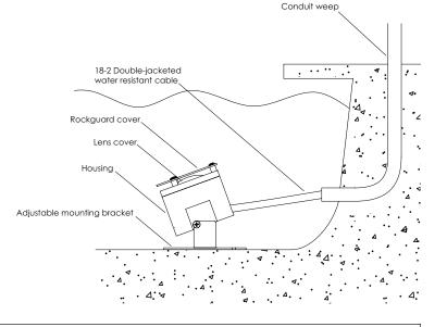
The operating voltage range for this LED luminaire is 6 - 15 volt AC. The Vista electronic driver ensures the LED operates at the intended lumen output while receiving voltage as low as 6 volts, and as high as 15 VAC, resulting in a balanced lumen output from the first fixture to the last. Eliminating the dimness issues often attributed to voltage drop.
