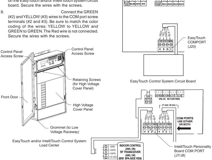
IntelliTouch Control System Circuit Board
