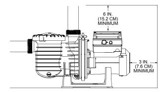
Figure 1: Pump Rear and Overhead Clearance
