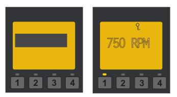
The pump will not run the scheduled speeds until the button is pressed (LED on) to place the pump in Schedule mode.
