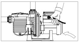
4. Reinstall the RS-485 communication cable.
