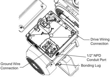
When the pump is started and stopped by removing power with a relay or timer, a two-pole device should be used to apply and remove power to both POWER LINE TERMINALS.
