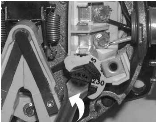
Figure 3: Changing the Voltage Setting
