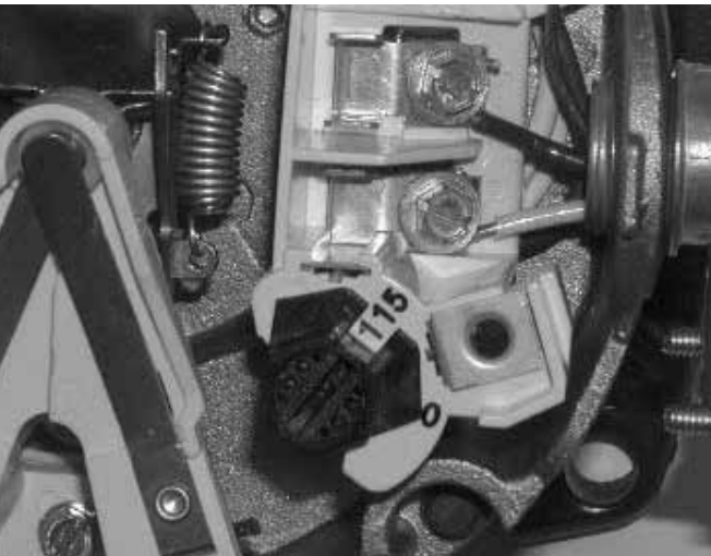
Figure 4: Motor Set for 115 Volt Operation
