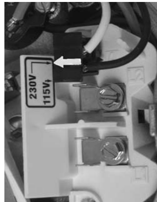
Figure 4A -Voltage Change Plug Set for 230 Volts
