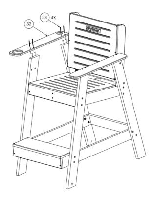
21.Install cup holder (27) using screws (34).
