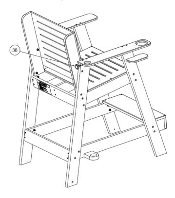
24.Install Anchor (39) using Bolt (33), Washer (36), and Nut (35).
