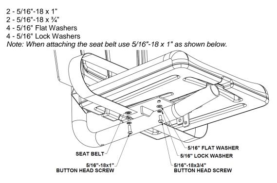
g. The below image shows the proper way to assemble the seat belt.
