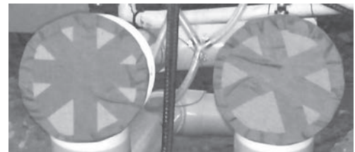
Figure 9 Taped Jet Housings
