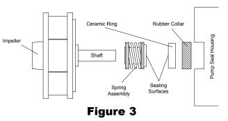
CAUTION: Do not damage the ceramic or carbon surfaces of the seal. If the surfaces is damaged, leaks will occur.
