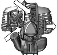
Dust and grass build up on the outside of the cylinder. This build up insulates the engine and prevents the heat from leaving.
