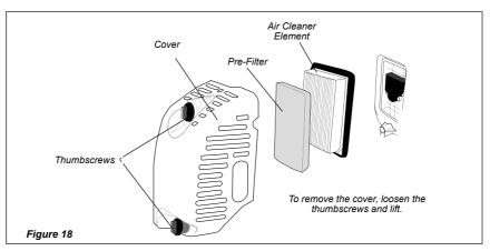
Install the filter element, pre-filter and cover in the reverse order of removal.
