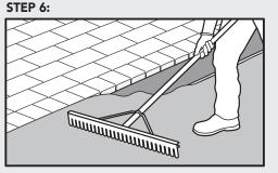
**Step 1:** Prior to compacting the pavers or natural stone, remove bedding layer (sand or chips) that extends outside the perimeter. For optimal performance, remove all of the bedding material down to the base material.
