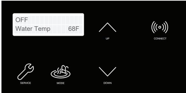
Figure 89. Wi-Fi Reset – Press and Hold CONNECT
