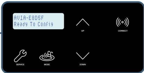
The CONNECT key displays the ID and connectivity status.
