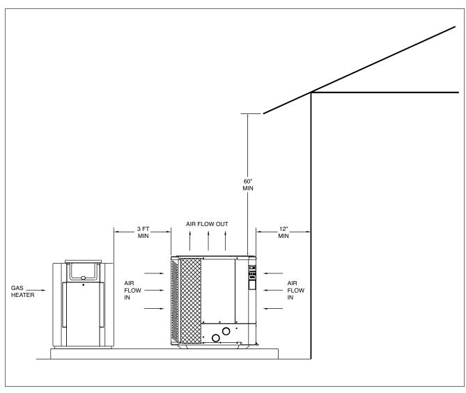
Fig. 1: Installation Clearances
