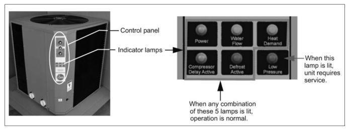
Fig. 3: Indicator Lamps — Analog Models
