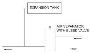
Figure 12. Air-Separation/Expansion Tank
