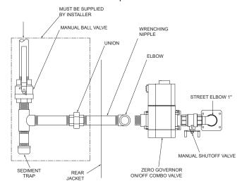
Figure 19. Gas Supply Connection
