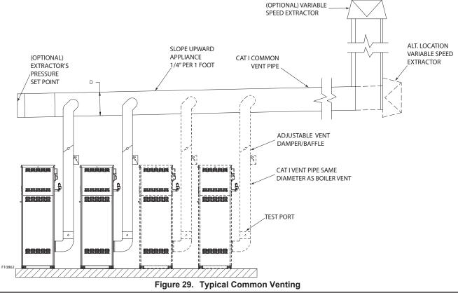
vent be less than the area of the largest heater exhaust outlet.
