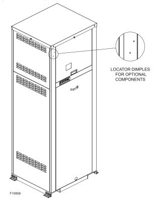
Figure 23. Locator Dimples for Optional Components
