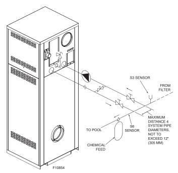
Figure 18. Single Pool Heater Application
