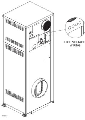
Figure 22. Wiring Location
