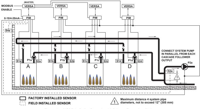
Figure 14. MODE 1 - Boiler Cascade with Primary/Secondary Piping
