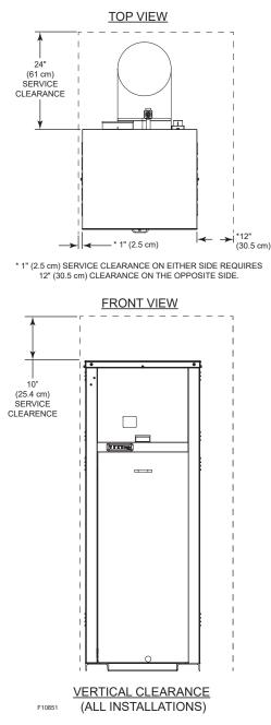
Figure 6. Minimum Clearances from Combustible Surfaces – Indoor and Outdoor Installations
