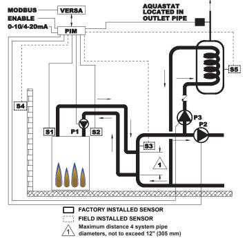
Figure 15. MODE 2 - Single Boiler with Indirect on System Loop
