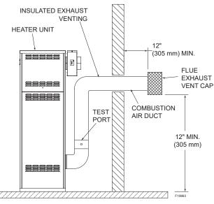
Figure 30. Horizontal Through-the-Wall Venting with Ducted Combustion Air
