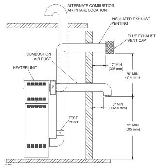
Figure 32. Horizontal Through-the-Wall Venting with Ducted Combustion Air
