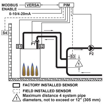
Figure 13. MODE 1 - Single Boiler with Primary/Secondary Piping
