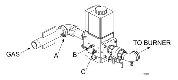
Figure 43. Gas Pressure Measurement Locations
