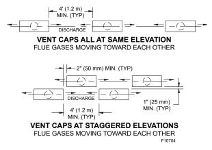
Figure 27. Vent Cap Configurations
