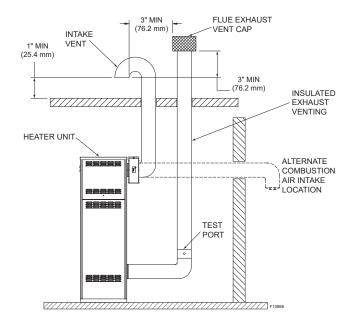
Figure 33. Vertical Vent with Ducted Combustion Air
