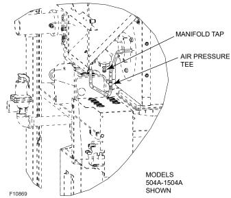
Figure 44. Air Pressure Tee
