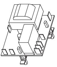
Figure 38. Low Water Cut-Off
