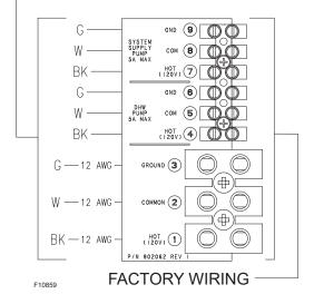
Figure 25. MVB Cascade Master Pumps
