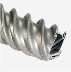
**SPIRAL TITANIUM TUBE** heat exchanger provides a corrosion-free waterway that can withstand the abuses of harsh pool chemistry. The spiral tube helps reduce deposit build-up and increases efficiency by performing a “scoop-and-lift” action.
