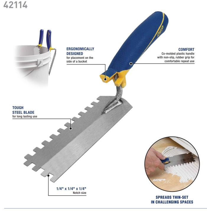
The QEP<sup>®</sup> 6" x 2" Comfort Grip Margin Trowel easily fits into mixing buckets and should be used to scoop and spread material, such as thinset and adhesive, in hard to reach areas. The non-slip, rubber grip reduces job fatigue for comfortable, repeat use. Crafted from tempered and hardened steel, this margin trowel is designed for long lasting use like underneath toe kicks and cabinets. The 1/4 in. x 1/4 in. x 1/4 in. notch size is for installing floor tile up to 8 in.
