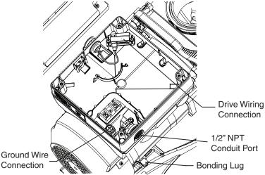
**Field Wiring Compartment**
