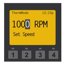
**Setting the Thermal Mode Pump Speed**
