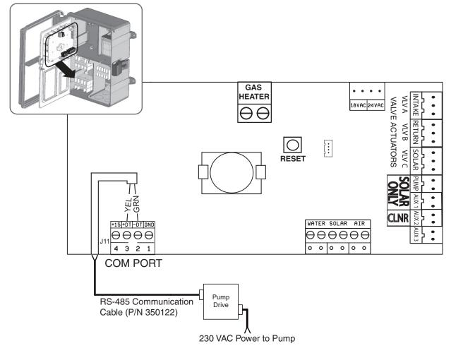
**SunTouch Control System Circuit Board**
