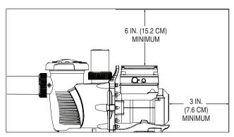
Figure 1: Pump Rear and Vertical Clearance
