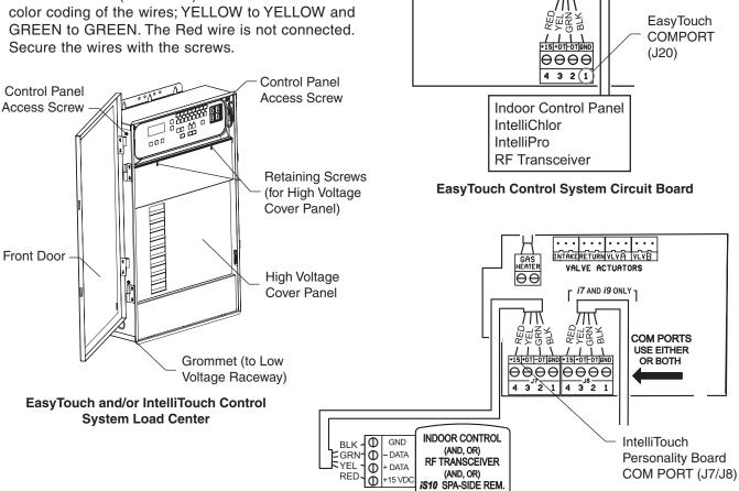
IntelliTouch Control System Circuit Board
