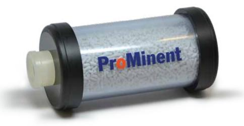
The **Acid Fume Separator (AFS)** is a proprietary device that allows for direct venting of an acid tank located inside a mechanical room. The **AFS** eliminates the need for costly venting via fans to outside areas or secondary water tank type fume traps. The result is a fume-free workplace with added protection of metal and electrical components. The proprietary reagent will change from white to purple when reagent is no longer effective.
