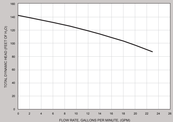
PB4-60 BOOSTER PUMP PERFORMANCE CURVES
