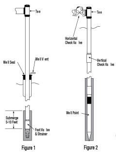
A shallow well system should not be installed where total suction lift exceeds 25 feet at sea level. Suction lift must be reduced at the rate of approximately 1 foot per 1000 feet at elevation. Total suction lift consists of the vertical distance from the water level when pumping to the pump plus losses due to friction in the pipe line. The volume of water delivered decreases with an increased suction lift.
