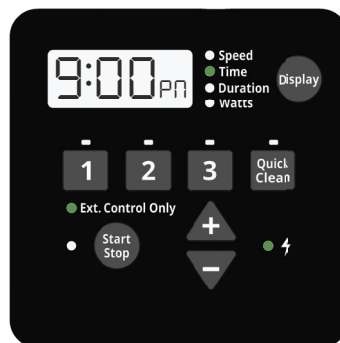
Figure 6: Activating External Control Only
