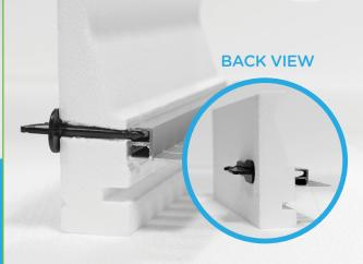
Rotate clip 90° vertically to lock it into the cover track.
