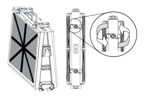
Reinstall the filters according to the diagram DO NOT FORCE THE FILTERS INTO PLACE.
