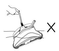
**Important:** Do NOT lift the robot pool cleaner from the water by its cable.
