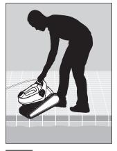
Please use the cable to pull the robot to the surface, then use the handle.
