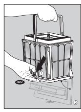
8.1.4 The debris can then be removed.
