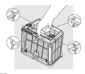
8.2.5 Assemble the filter panels according to the following order: Panel  $4 \rightarrow 3 \rightarrow 2 \rightarrow 1$ .
