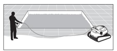
5.1.2 Unwind the blue cable and stretch it out completely so that it has no kinks.
