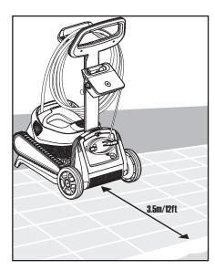
5.1.1 Position the power supply so that it is approximately in the middle of the long side of the pool at a distance of 3.5m/12ft.
