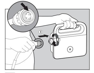
**5.1.3** Attach the blue cable to the power supply by inserting it with the notch on the connector (1) lined up to the groove in the socket on the power supply. Turn it clockwise (2).
