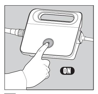
5.2.2 Turn the power supply ON. The Pool Cleaner will now operate until it has reached the end of the cleaning cycle.
