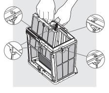
8.2.1 Hold down the handle to remove the inner net basket.
