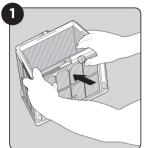
Dismantle the panels, starting with pressing on panel no.1 using your thumbs.
