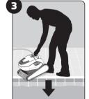
Put the Pool Cleaner into the pool Release the Pool Cleaner and let it sink to the floor of the pool. Make sure that the floating cable is free of any obstructions.
