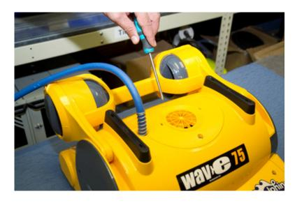
Remove screw(s) holding impeller cover in place.
