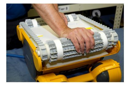
Snap new brush into place by aligning brush under the tracks and firmly rolling it forward until it clicks in place.
