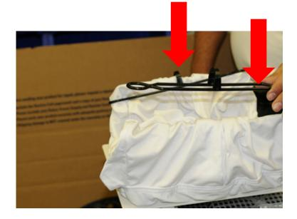
To remove the filter bag, remove black plastic clips and slide bag off of metal frame.
