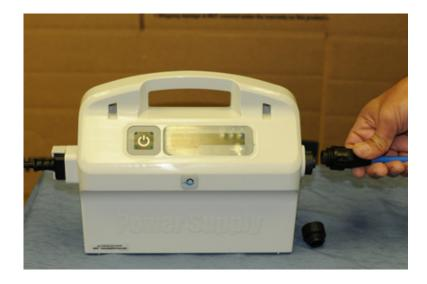
Plug other end of cable into power supply and turn the power supply on.
