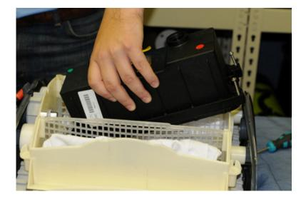
The entire motor unit easily comes out and can be replaced with a new one.
