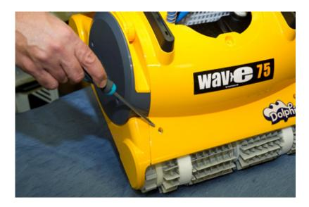
Remove the 4 screws (2 per side) that hold the robot cover to the chassis
