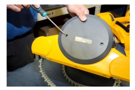
With cover and brushes removed, remove the 2 screws holding the side panel in place.
