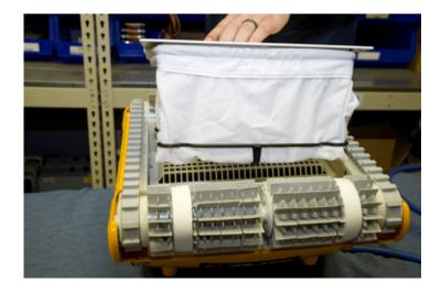
Remove the bottom lid. The filter bag will be attached to the lid on a metal frame.
