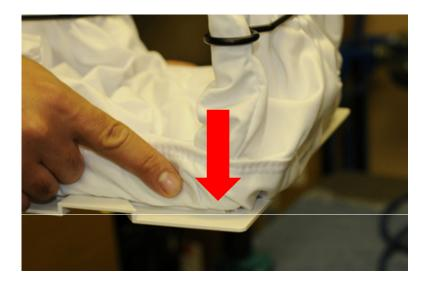
When putting filter bag back in place, ensure that the elastic band is completely down over the lip at the base of the bottom plate to prevent dirt and debris from escaping bag.
