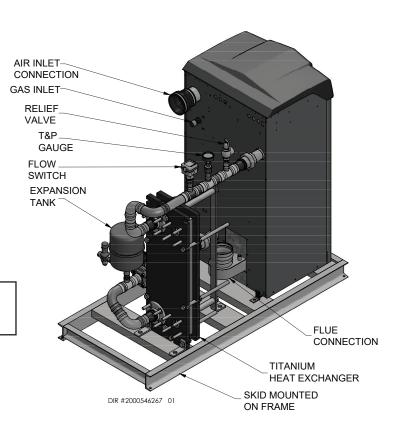
RECOMMENDED CLEARANCES: BOILER - SEE FTXL I & O MANUAL INDIRECT HEX - ALLOW 18" FOR SERVICE ON ALL SIDES
