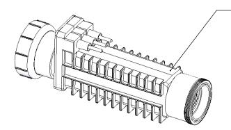
CC15-MF: CC15 Replacement Cell Male/Female Unions (Commercial) for Multiple Cell Manifolds
