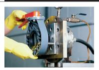
Colonial Butterfly valve are tested under high pressure for structural integrity and low pressure for a bubble-tight seal.
