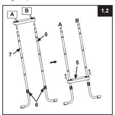
**IMPORTANT:** Ensure the J-shaped legs are pointing outwards before installing the steps.
