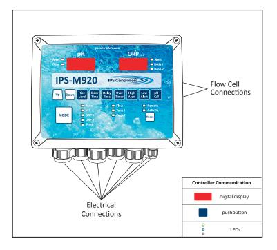
Figure 2: M920 Controller Components Connections
