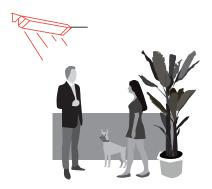
Angle fixture 30° to 60° from horizontal face down. Best angle is approximately 45°.
