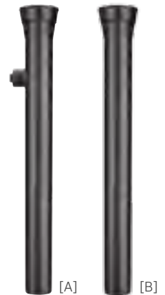
[A] PROS-12-SI [B] PROS-12 Retracted height: 16 1/8" Pop-up height: 12" Exposed diameter: 2 1/4" Inlet size: 1/2"
