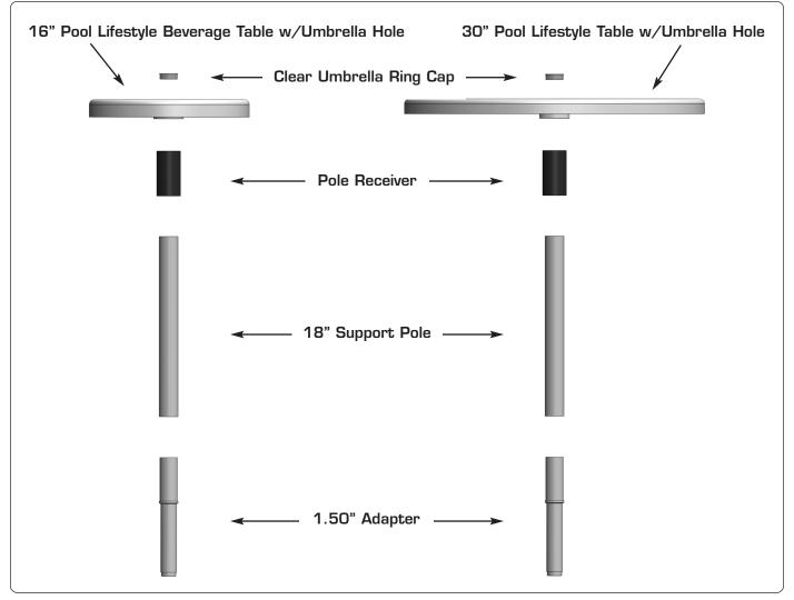
**Figure 1:** 30" PL Table w/Umbrella Hole, Pole Receiver, 18" Support Pole, 1.50" Adapter; 16" Beverage Table w/Umbrella Hole, Pole Receiver, 18" Support Pole, 1.50" Adapter
