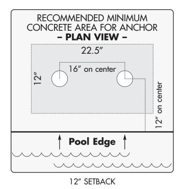
RECOMMENDED MINIMUM CONCRETE AREA FOR ANCHOR PLAN VIEW -22.5" 16" on center center O င်္ **Pool Edge**
