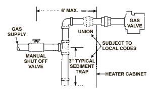
Figure 21: Sediment Trap
