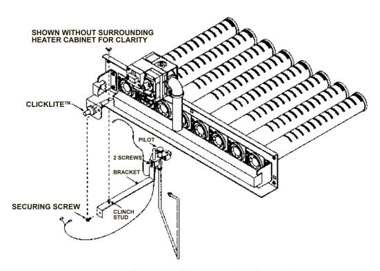
Figure 48: Pilot Assembly Removal
