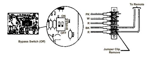
Connection to 2-wire Remote On/Off Switch
