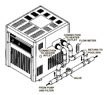
Figure 24: Manual By-pass Valve
