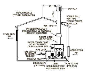
Figure 16: Vent Top Installation
