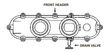
Figure 42: Drain Valve Location
