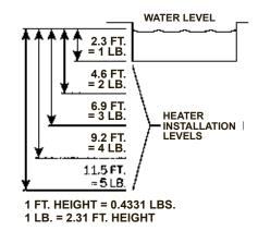
Figure 37: Heater Installation Below Pool
