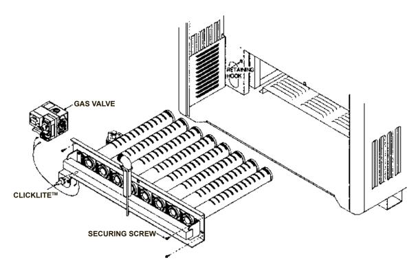
Figure 47: Burner Removal
