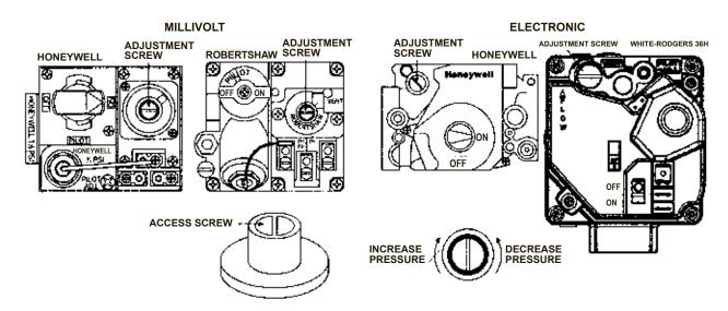
Figure 36: Valve Adjustment Screw
