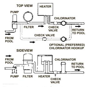
Figure 28: Automatic Chlorinator
