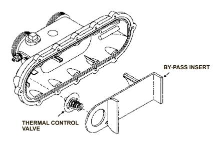
**Figure 55: Thermal Control Valve**
