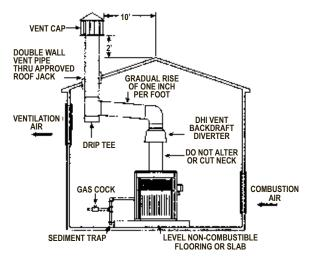
Figure 17: Indoor Installation
