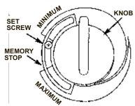
Figure 41: Temperature Controls
