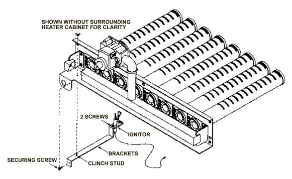
Figure 49: Ignitor Assembly Removal
