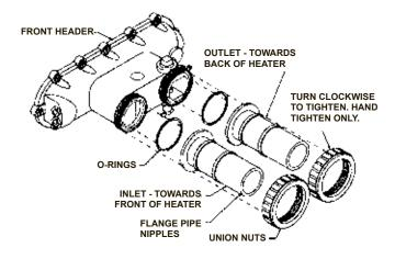
Figure 22: Pipe Nipple Installation
