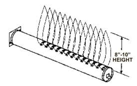
Figure 45: Main Burner Flame Characteristics
