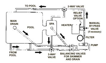
Figure 25: Typical Plumbing To Pool
