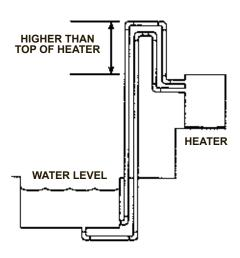
Figure 27: Heater Installation Above Pool
