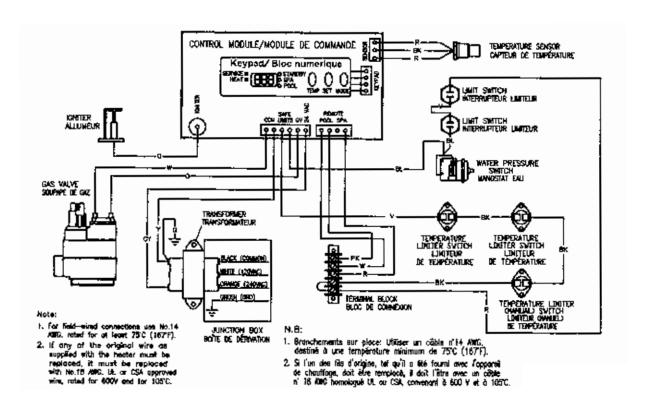
Figure 33: Wiring Connection Diagram
