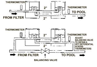
Figure 26: Multiple Heater Hookups
