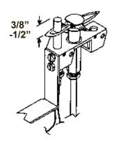
Figure 46: Pilot Flame Characteristics
