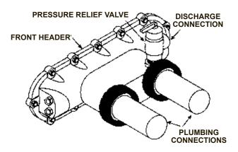
Figure 29: Pressure Relief Valve
