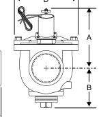
Operating Pressure:2 to 200 PSIMaterial:Cast Iron and BroEnd Connections:NPT (BSPT OptioVoltage Operating Range:22-28 VACLow Current Requirement:0.40 A at 24 VACAssembly:Valve comes fullyOptional:Purple Handle forOptional:Epoxy Coating
