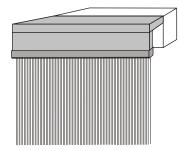
AQUA RAIN Part # G A 0 3 \_\_\_\_\_ 48 OR 64 STREAMS PER LIN FT. 2 ROW VERTICAL WATER DIRECTION RATE: 1/2 OR 2/3 G.P.M. PER INCH REMOVABLE NOZZLE INSERTS FOR DEBRIS AQUA SHOWER Part # G A 0 2 48 OR 64 STREAMS PER LIN. FT. 2 ROW HORIZONTAL WATER DIRECTION REMOVABLE INSERTS FOR DEBRIS RATE: 1/2 OR 2/3 G.P.M. PER INCH AQUA SPRAY
