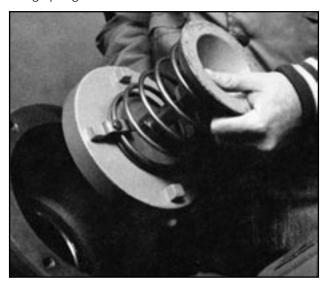
a. Un-thread retaining nut from stem and remove disc washer and seat disc.
