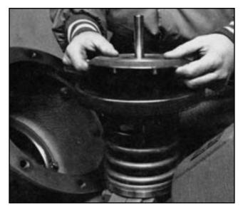
b. Inspect seat disc for wear or damage. Replace with new seat disc or turn used disc over if new disc is not available.
