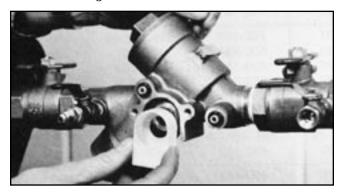
c. Carefully place the relief valve body over the bushing and tighten the two capscrews to retain the relief valve body to the main valve body. New capscrew sealing washers should be installed to avoid leakage.
