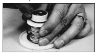
e. To remove spring and/or main stem from the guide, keep unit compressed and remove the screw (item 18) located in the center of the button. Push the main stem through the guide and remove the o-ring from the main stem. Inspect and clean or replace o-ring and seat disc as required. Clean all parts thoroughly with clean water before reassembly.
