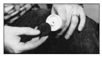
NOTE: The seat discs are symmetrical. It is usually possible to turn the disc over and obtain an effective seal.
