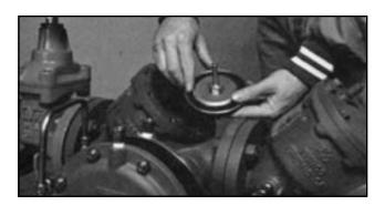
c. If the seat disc has been severely cut along the seat disc ring diameter, the assembly is being subjected to extremely high back pressure from thermal water expansion, water hammer, or other causes of excessive water pressure. A disc damaged in such a manner should be replaced and not turned over to be reused.
