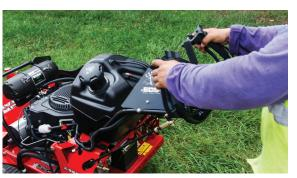
**PATENTED ENHANCED CONTROL SYSTEM** With Exmark's ECS, all the primary controls are close at hand for increased convenience and maneuverability. The design places hands in a protected position, where they're less likely to get banged up by branches and shrubs. Best of all, this natural, ergonomic hand position helps reduce operator fatigue.
