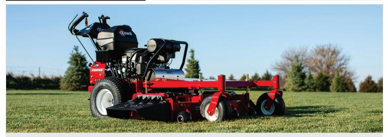
The Turf Tracer<sup>®</sup> is Exmark's premium wide-area, walk-behind mower, combining the productivity of larger cutting decks and hydro-drive components with the unmatched quality of a full-floating deck. They are engineered for speed, efficiency, and durability, and always deliver a quality of cut that is second to none.
