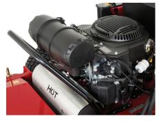
**SUPERIOR AIR FILTRATION** All X-Series models have a heavy-duty canister air filtration system for longer engine life, more efficient performance and simpler maintenance.
