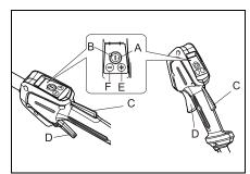
Hold down trigger switch 3. lockout (C) and depress trigger switch (D) to increase RPM to operating speed.
