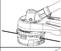
Hold trimmer head while turning knob clockwise to wind line onto spool until about 13 cm (5 in.) of each line remains exposed.
