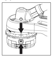
Insert one end of trimmer line into an eyelet, and push line equal distance through trimmer head.
