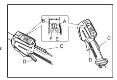
3. Hold down trigger switch lockout (C) and depress trigger switch (D) to increase RPM to operating speed.
