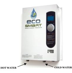
Once both water lines are fastened and secured you MUST run water through the unit for at least 2 minutes to FLUSH any air pockets (purging) in the lines, it is recommended that all faucets, showers etc be run. Failure to follow this step can cause permanent damage to the unit. This procedure MUST be performed before any electrical power is turned on.
