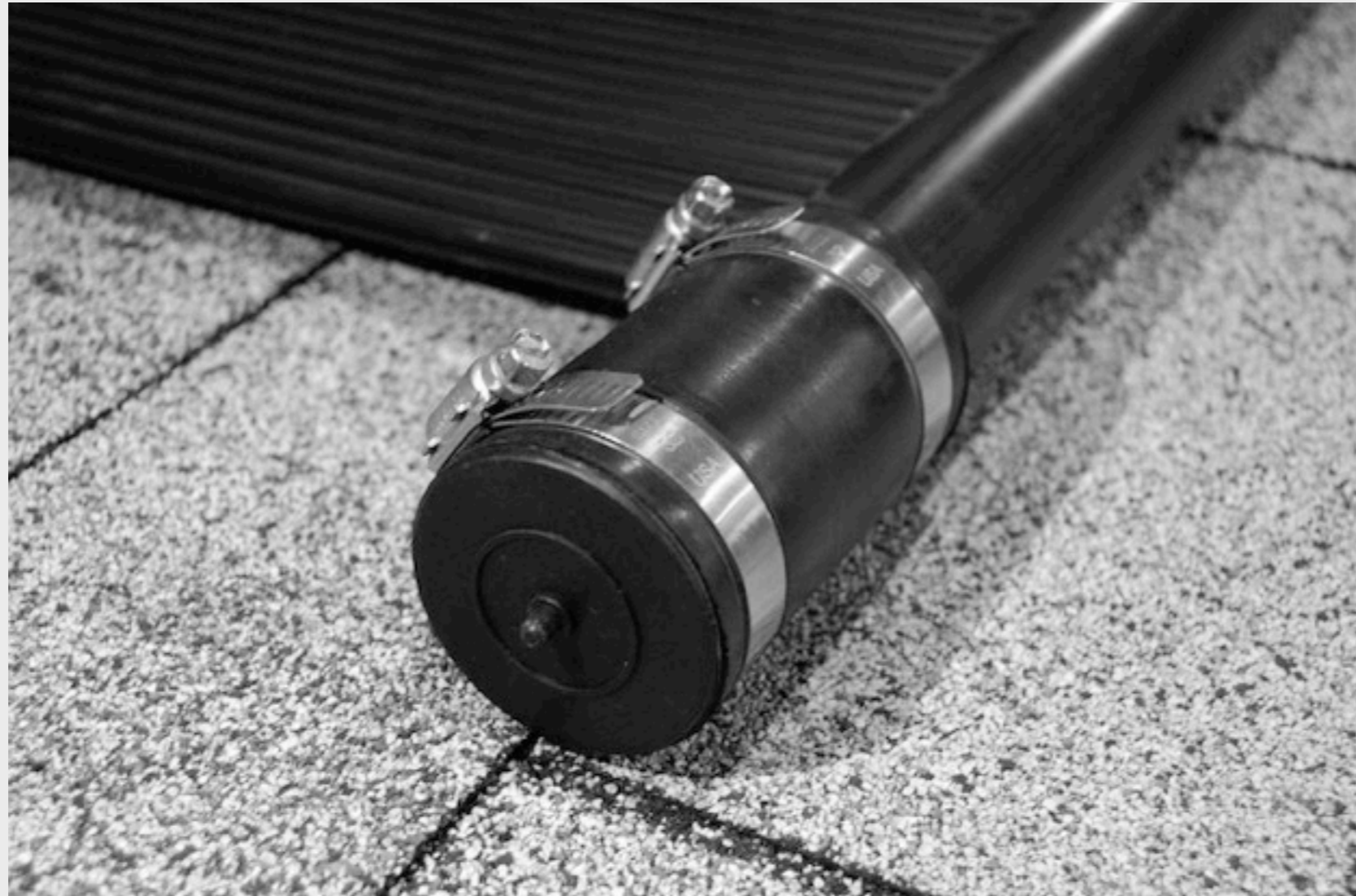
FIGURE 11 Installed End Cap
