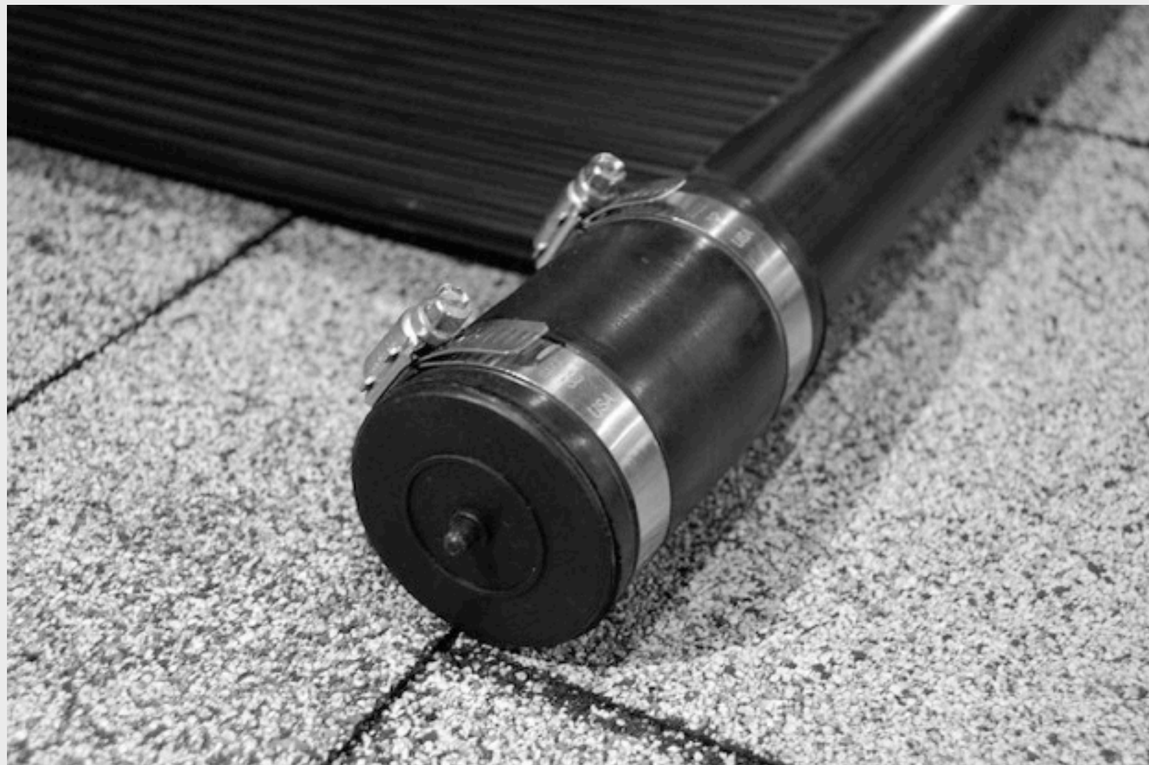
FIGURE 11 Installed End Cap
