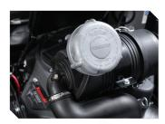
**Turbinator Pre-Cleaner** – Exclusive feature removes debris for cleaner air
