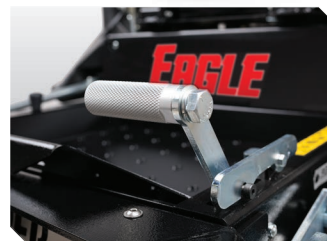
OCDC - Foot-operated to keep your hands on the steering levers
